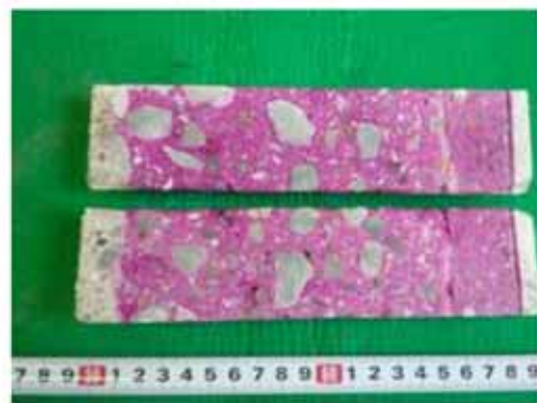
●中性化深さ測定状況
